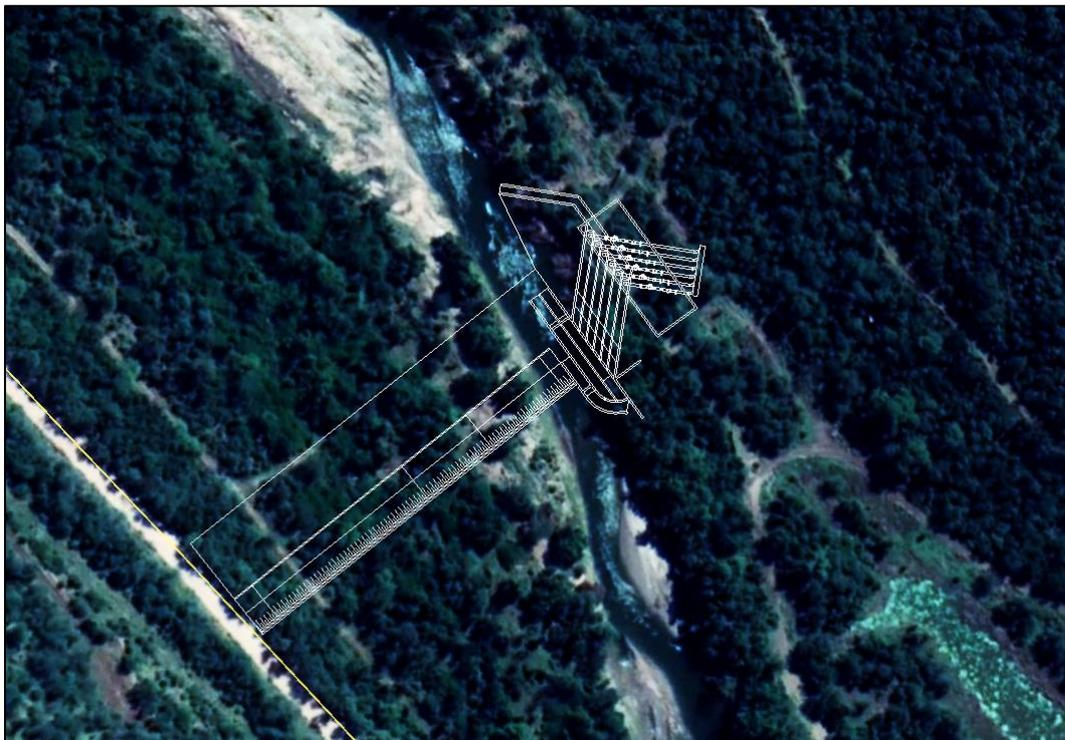
Figure 7-1: Overlay of proposed weir structure ( $\pm 4 - 6$  m high) over Crocodile River at site CROC4
