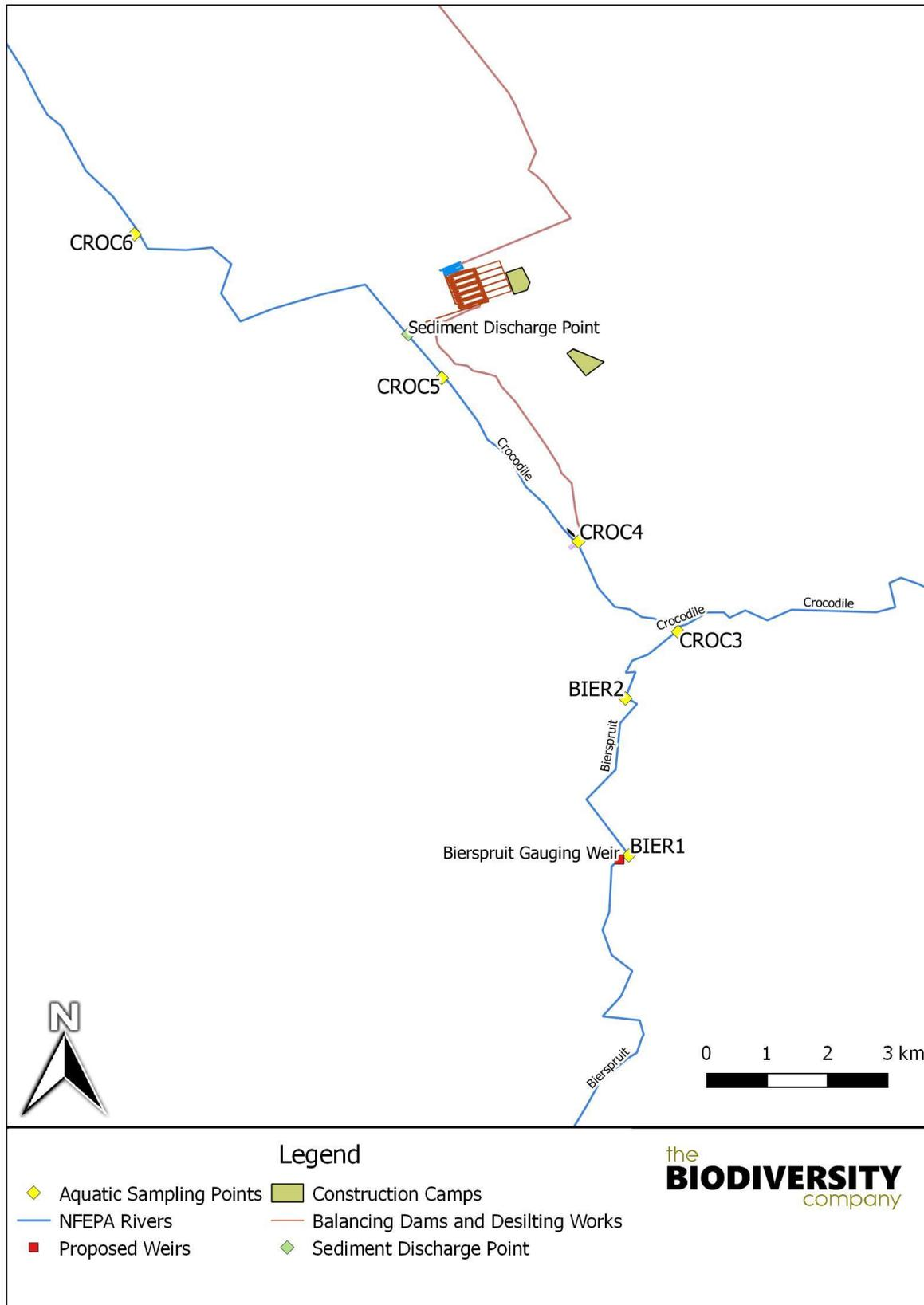
Figure 2-5: Illustration of the Bierspruit Gauging Weir, abstraction weir and sediment discharge point and aquatic sampling points
